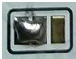
There is a healthy-sized solder blob over two pads, allowing current to flow from the center pad to the pad on the left side. The third pad (on the right) has no connection to the other two pads.
