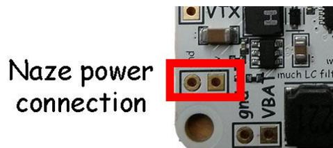
Two female round pin headers will be used in this connection. The male pin headers will be inserted into the ground and +5V connections on the "Motor 6" connection on Naze.
